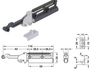
For groove mounted and concealed runners with gap width S 3 - 6 mm
